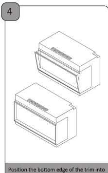
Position the bottom edge of the trim into the opening of the fire until it rests in front of the glass. Then push the the top edge inwards. Gently push all four corners of the trim to ensure a snug fit.
