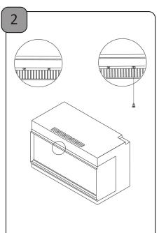
Identify the screw detailed above, located in front of the heater outlet grill, and remove it. Keep aside for later.
