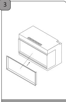
Offer the trim to the fire, ensuring the correct orientation - the top of the trim has a shallower return than the bottom.
