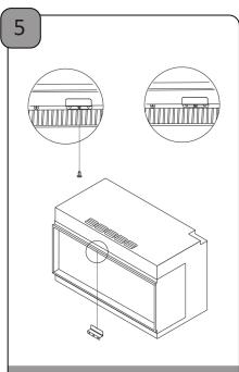
Take the small trim bracket and secure it to the fire using the screw removed earlier. The bracket is used to hold the centre of the trim up, not pull it towards the fire.
