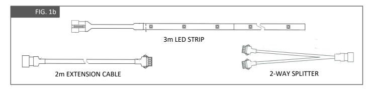
The length of an individual kit may be extended by joining another kit using LED strip connectors (not supplied), but only to a maximum of the appliance loadings, see table below for details.
